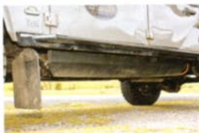
Above left: the sills hide two auxiliary tanks for water and diesel; above right: the central storage area
