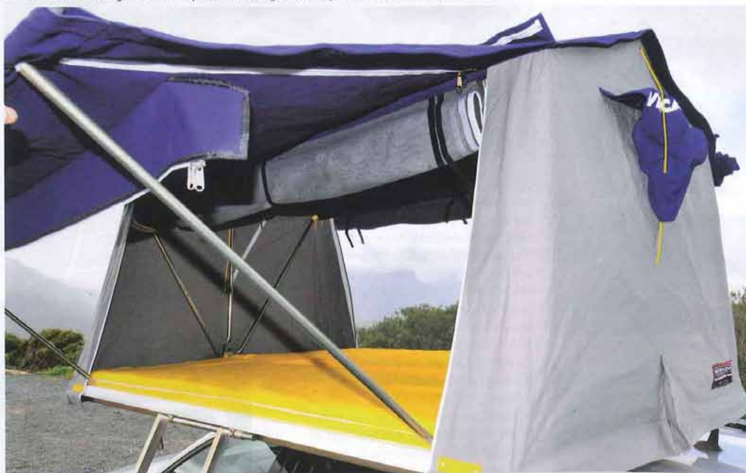
Left: The floor platform is hinged in the middle. Right: You secure the waterproof cover by pulling the elastic cord over the clips. Below: The small rectangular window flaps (seen on the right) can be opened or closed from inside the tent.
