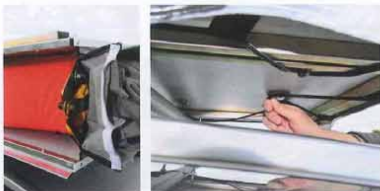
Left: The floor platform is hinged in the middle. Right: You secure the waterproof cover by pulling the elastic cord over the clips. Below: The small rectangular window flaps (seen on the right) can be opened or closed from inside the tent.
