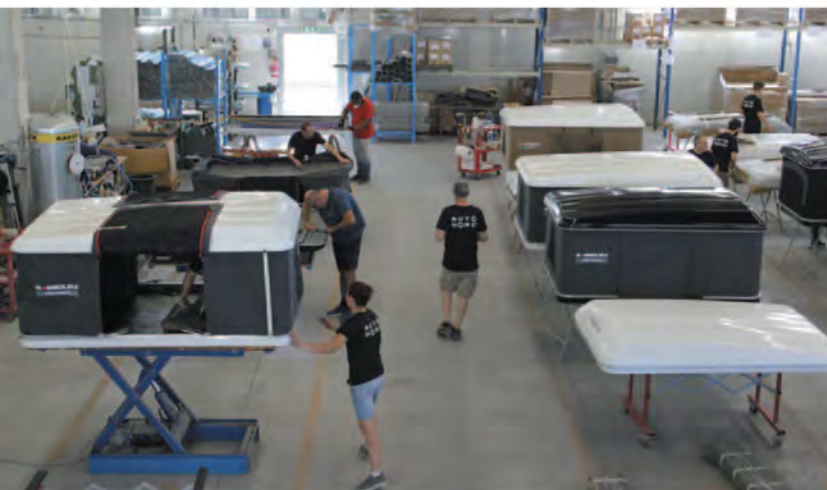
The assembly of the tent on the fiberglass shells, that comes from the molding is manual.
