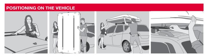
The exclusive Autohome fixing system, with 2 "C" guide rods in the base, allows the tent to be fitted to any vehicle roof: family car, off-road, station-wagon with railing, SUV, camper, van, pick-up, sheeted vehicle, truck... Quick and safe, the system has 4 adjustable clamps – a standard feature – to position and secure the tent as required on any roof or railing, without risk and without needing to change the bodywork.
